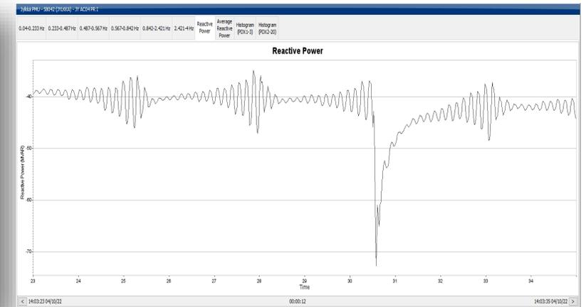
Jylkkä 400 kV active and reactive power measurements
