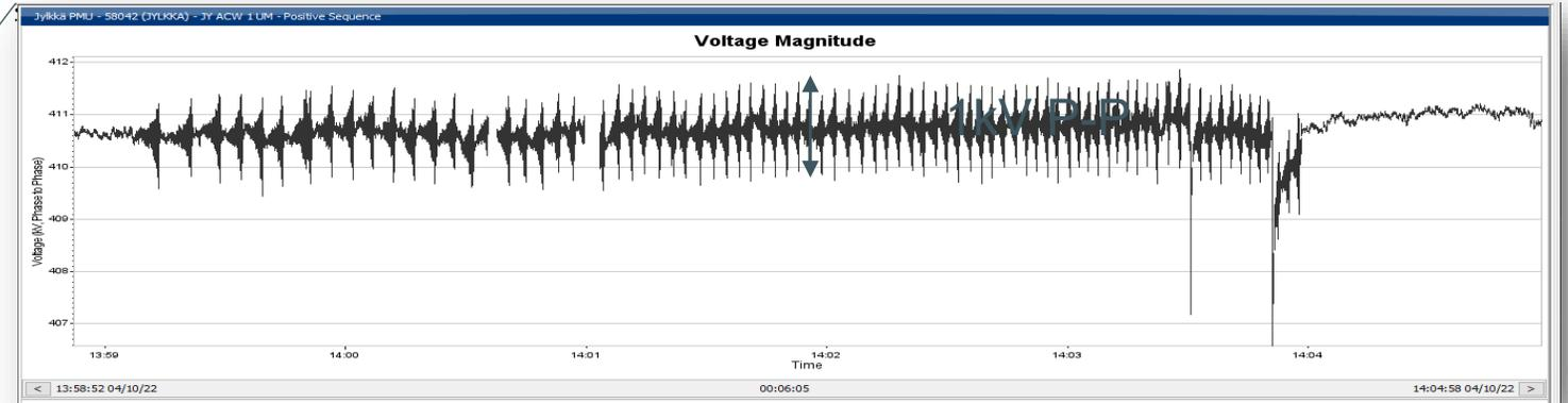
Jylkkä 400 kV voltage PMU measurement
